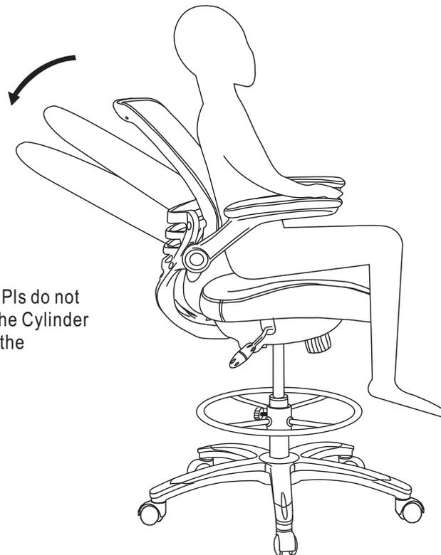
**Attention:** Be careful! Pls do not use tilt function once the Cylinder Column is adjusted to the topest height.
